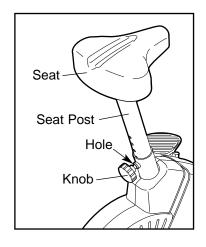
Next, slide the seat post up or down and align one of the adjustment holes in the seat post with the indicated hole in the Frame. Insert the knob into the frame and the seat post, and turn the knob clockwise until it is tight. Make sure that the knob is inserted through one of the adjustment holes in the seat post.
